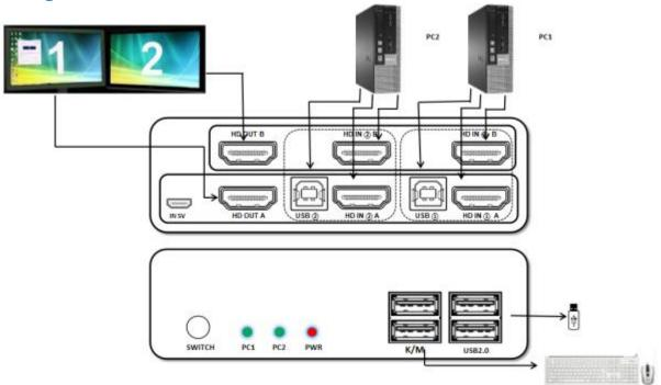
(Note: Please note that in the premise that the host computer supports multi-screen display, the extended mode can output two different screens, and the copy mode can output two identical screens; if the computer only supports single-screen display, even if there are many One output port, only one output port works when the wiring is correct.)
